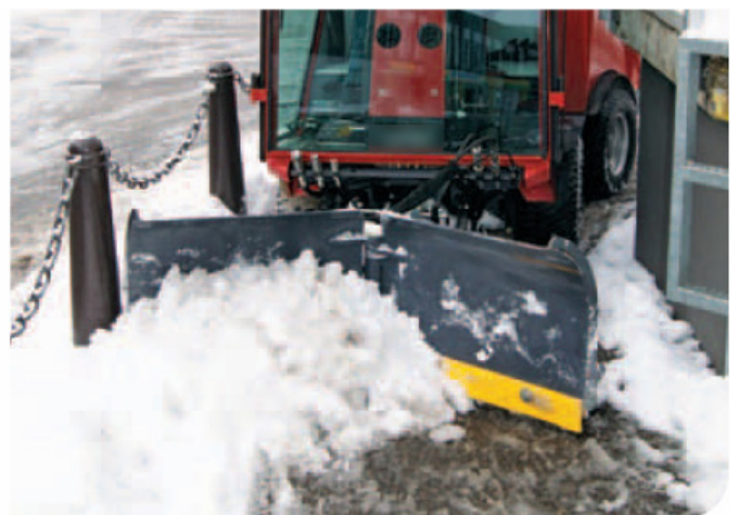
The V-Blade has three modes: left or right angled, V-shaped outwards and V-shaped inwards to collect snow
